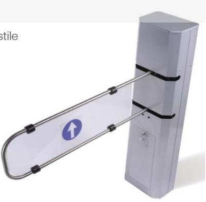
**Saloon** is a bidirectional through-way that works with clearing signals in both directions. Its control electronics open the gate-leaf in the chosen direction on a time-by-time basis. The clearance signal, which is received by a card reading device or other device, activates the motor in the respective direction of rotation.
